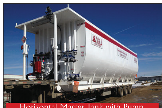
Horizontal Master Tank with Pump Manifold mounted on the porch
